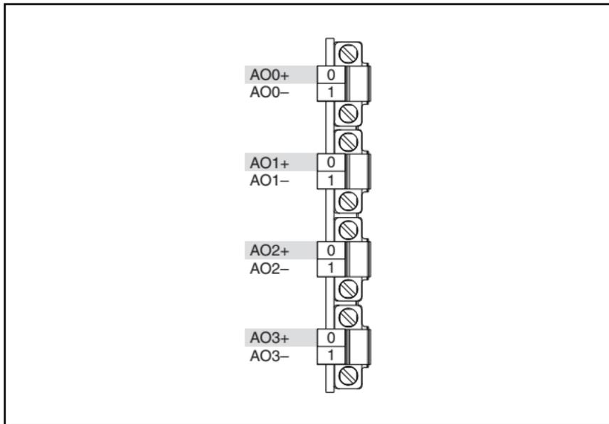
**Figure 2.** NI 9269E Terminal Assignments
