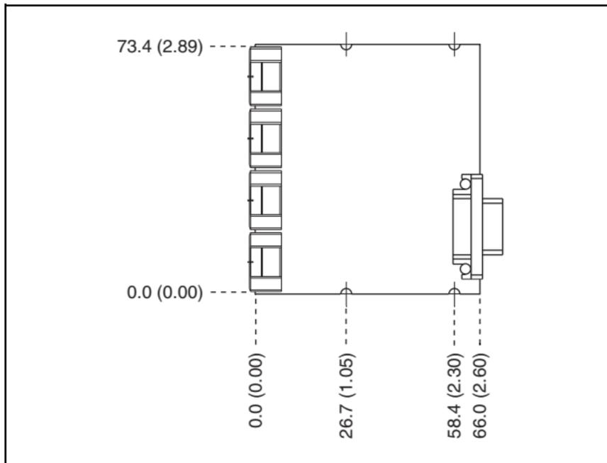
**Figure 1.** NI 9269E Dimensions in Millimeters (Inches)
