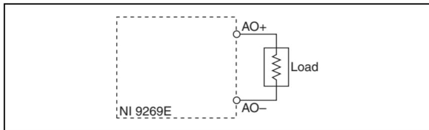
**Figure 3.** Connecting a Load to the NI 9269E
