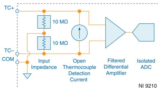
The channels of the NI 9210 share a common ground isolated from other modules in the system. Each channel passes through a filter and then a 24-bit analog-to-digital converter (ADC) samples the channel.
