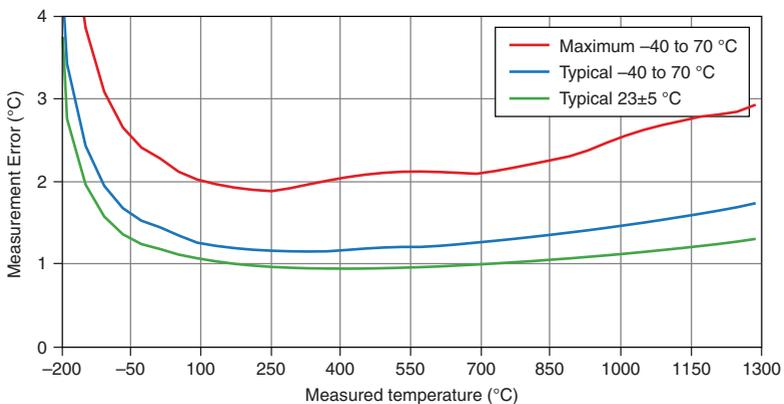
**Figure 3. NI 9210 with Mini-TC Thermocouple Type K Errors**
