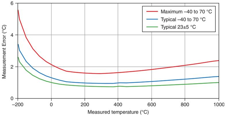
**Figure 7. NI 9210 with Mini-TC Thermocouple Type B Errors**
