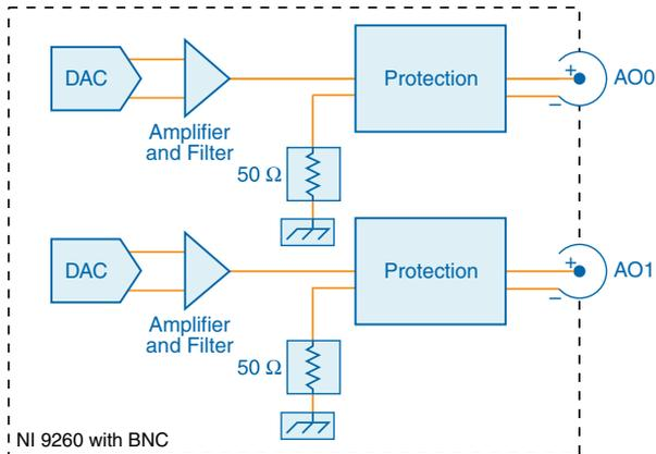
The Delta-Sigma DAC has a resolution of 24 bits and can update at a maximum rate of 51.2 kS/s. The output stage of the NI 9260 with BNC is pseudo-differential. AO- is terminated using a 50 Ω resistor to GND.
