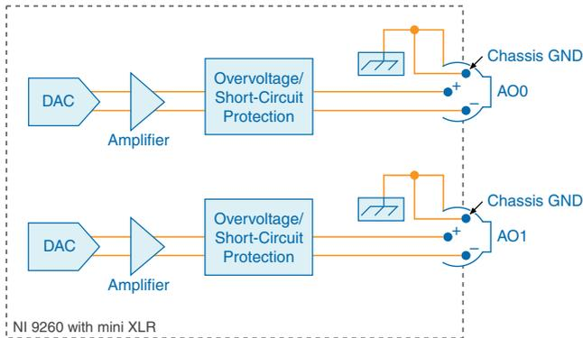
The output stage of the NI 9260 with mini XLR is balanced and fully differential. The AO- pin represents one output of the differential output driver and is capable of driving signals into the minimum load. Connecting this pin to GND will short circuit the output.
