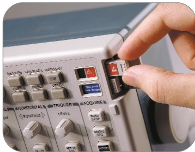
► Application module being installed.
